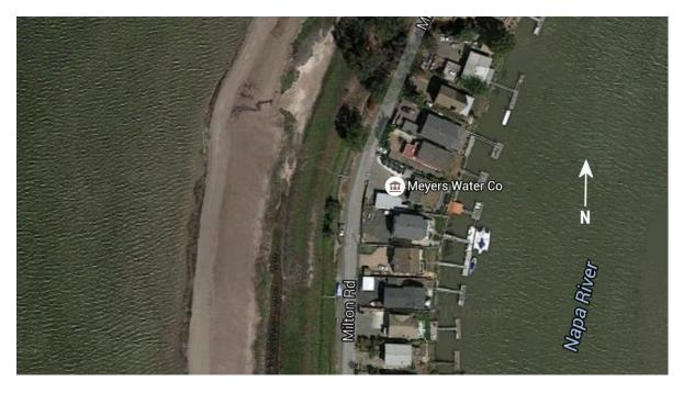
High tide waters push into the slough on the west side of the development; there is only a partial levee protecting the west side. The Napa River abuts against the levee on the east side.
